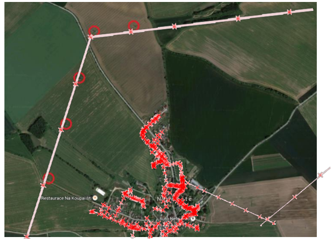
Figure 4 – Ortophoto map of Nedeliště with marked 22kV electricity pylons and above-ground powerlines [Source: Google Earth with the application QGIS]
