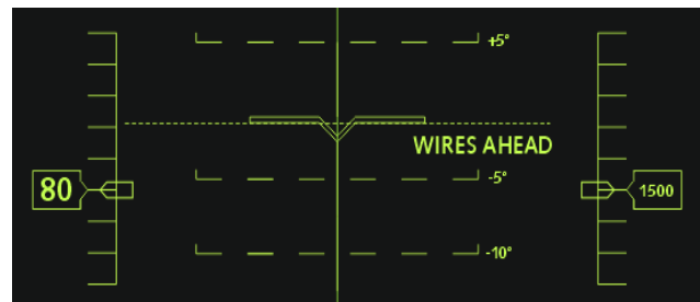
Figure 5 – HUD projection of WIRES AHEAD warning
