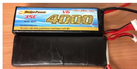
Figure 3 – View of the lithium-polymer battery used to power the airscrew propulsion
