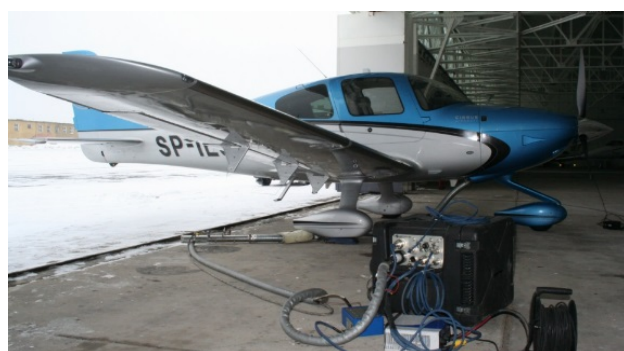
Figure 7 – Location of the exhaust gas intake probe during the tests
