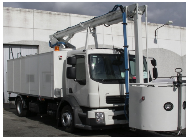
Figure 2 – A device for de-icing and protecting aircraft against icing
