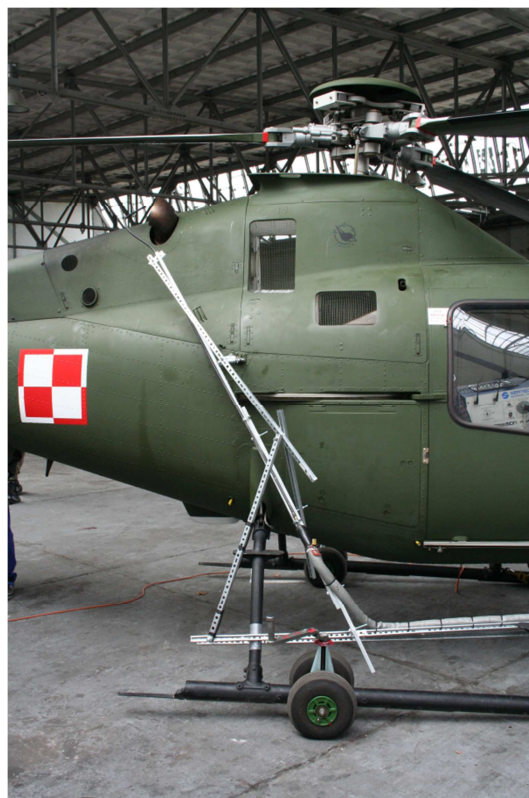
Figure 3 – Placement of the exhaust gases probe
