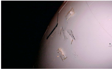
Figure 1 – Typical ground handling damage
